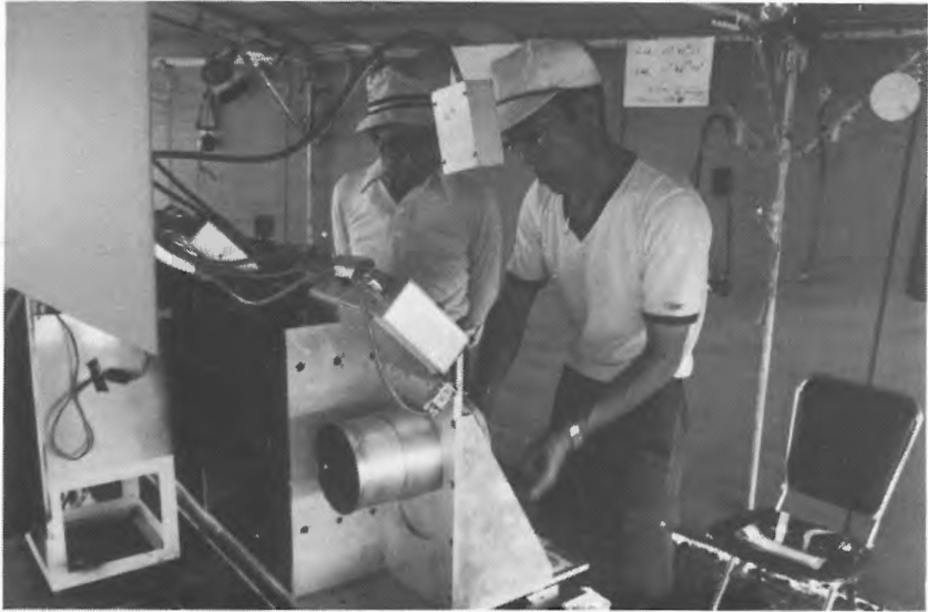
Fig. 1(2). Camera part of horizontal telescope.
